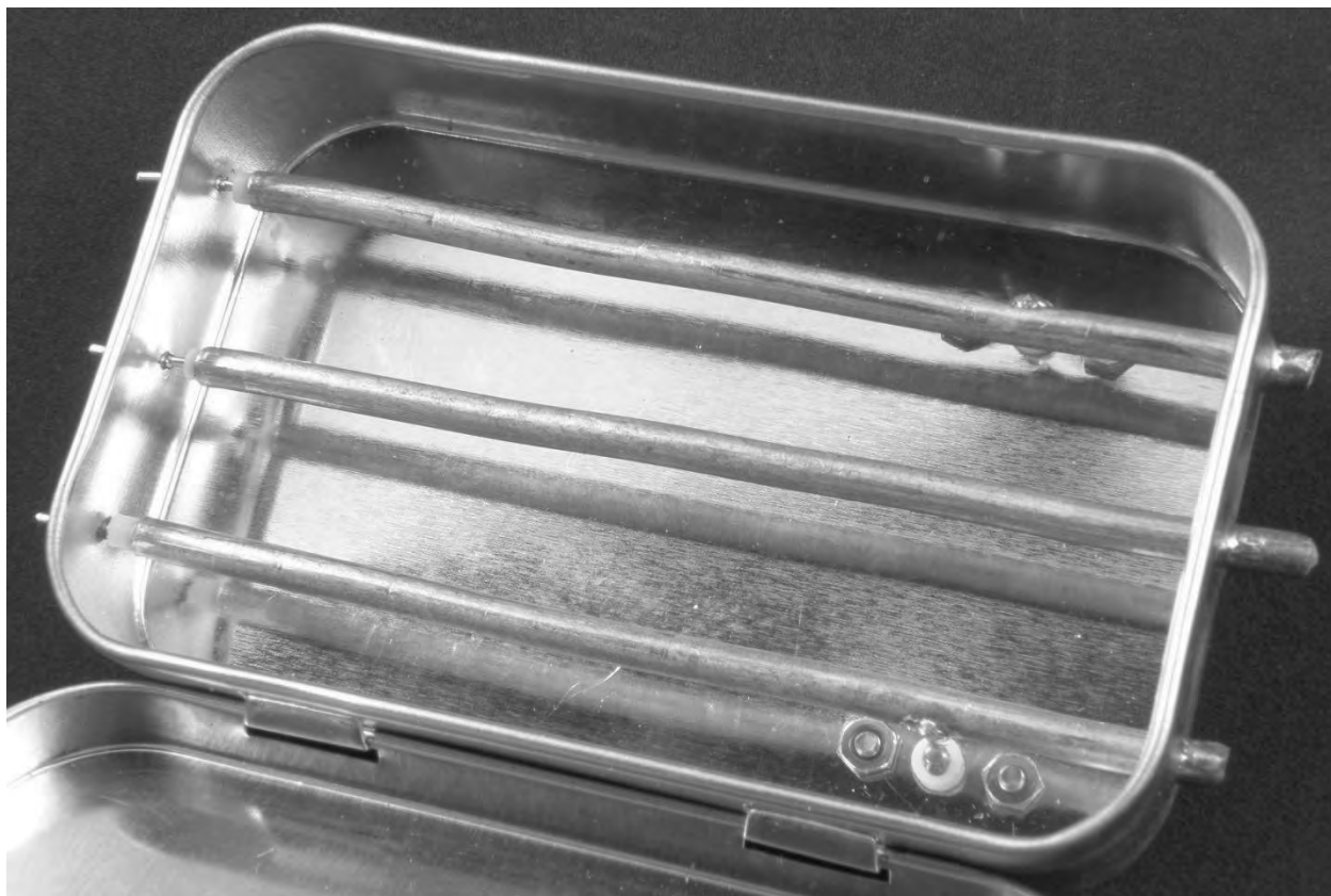
Figure 1 – 432 MHz Combline filter in Altoids tin
