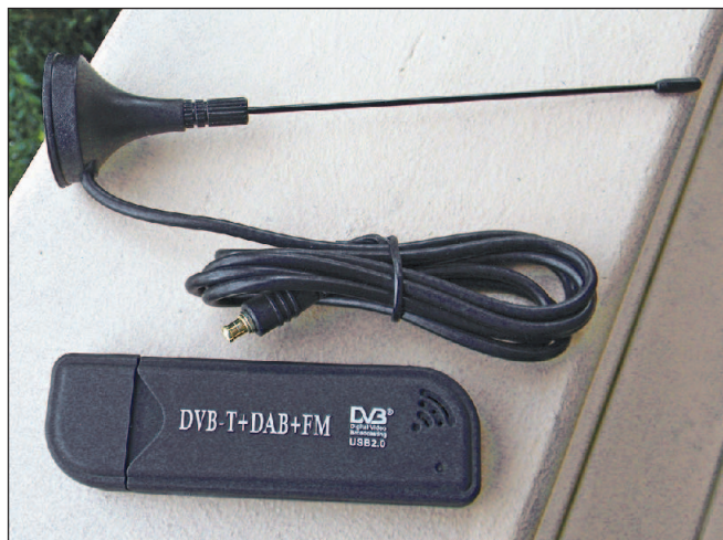
Figure 1 — Purchase a dongle that includes the small whip antenna. Cut and use the supplied cable and connector to save cost and assembly time.
