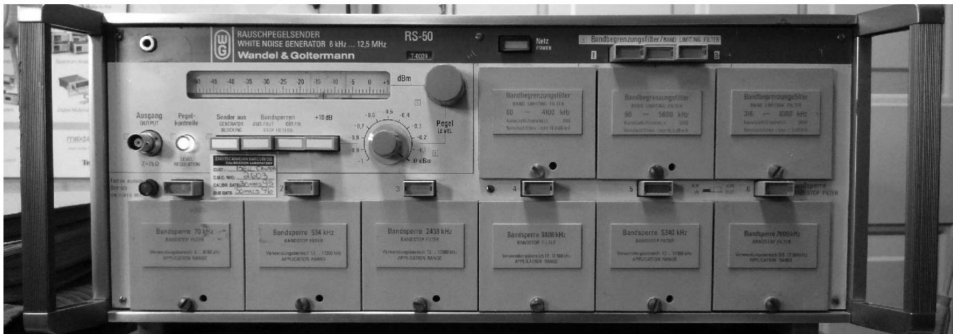
Figure 5 — The Wandel & Goltermann RS-50 white noise generator.
