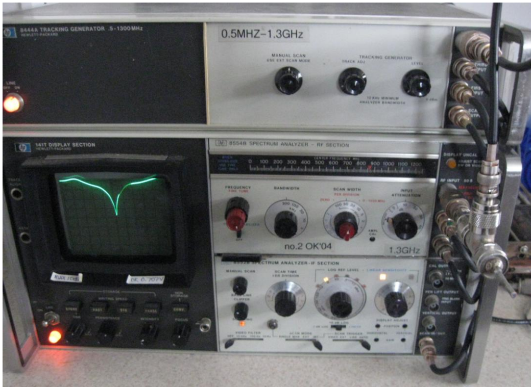
864 MHz 1/4 Wave Coaxial Notch Filter Performance. 10dB per Division Vertical, 50 MHz per Division Horizontal.
