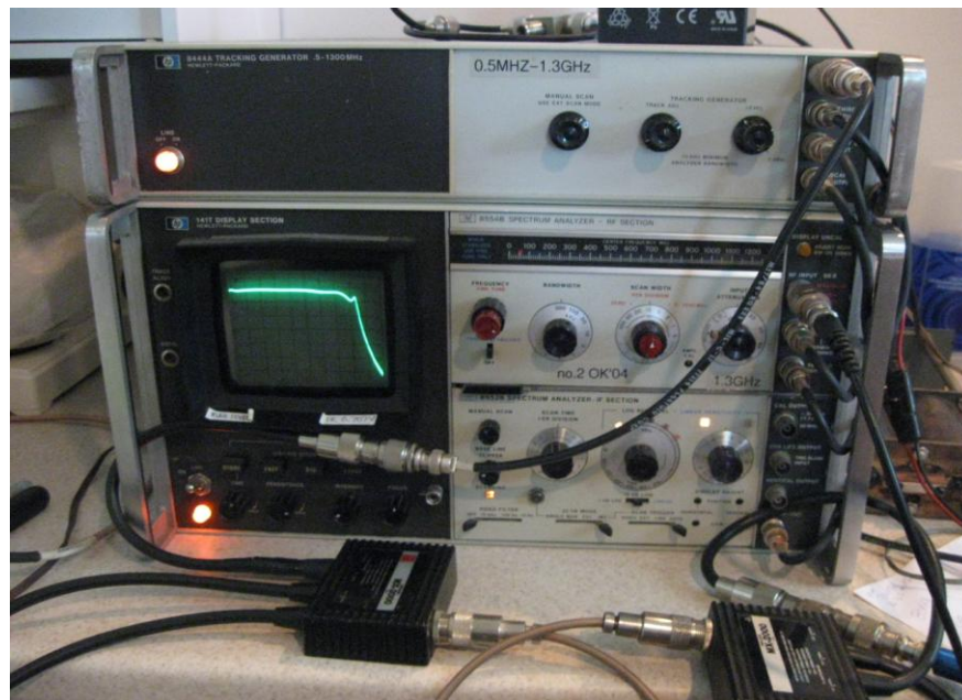
Back-to-Back Diplexer Configuration Showing 60dB Notch at 100MHz. View Centered on 50MHz, 10MHz per Division Horizontal and 10dB per Division Vertical.
