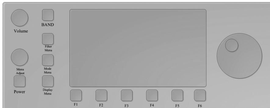
Figure 1 — Here is my proposed front panel layout for a self contained SDR. The display panel has 800 × 480 pixels, to give a full color internal computer display of control functions and data. The menu keys along the left have dedicated functions and the keys along the bottom are soft function keys.
