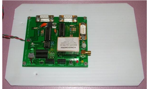
This near space tracker is one of my kits. You can also use a TNC and HT.
