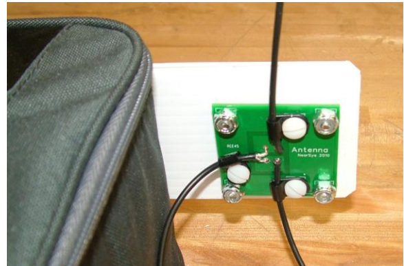
The antenna after it's been attached to the Antenna Boom. This is a circuit board of my design that I use for making near space dipole antenna.
