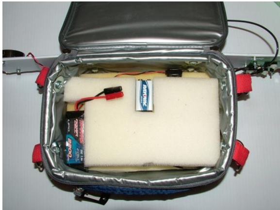
The battery on the left is a 2-cell, 25C, 2200 mAh rechargeable lithium battery. The battery's original connector was replaced with an Anderson PowerPole connector. The 9 V battery is for an audio beacon mounted to the Antenna Boom.
