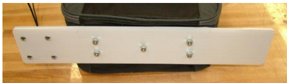
The antenna boom is very lightweight, so three small screws are sufficient to hold it into place (the five screws in this image are overkill).
