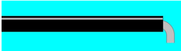
Very little of the #12 AWG wire needs to be stripped and bent. This is where it will be soldered to the perforated board.
