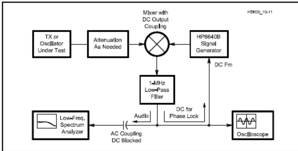
**Figure 3 — Arrangement for measuring phase noise by directly converting the signal under test to audio. The spectrum analyzer views the signal’s noise sidebands as audio; the signal’s carrier, converted to dc, provides a feedback signal to phase-lock the Hewlett-Packard HP8640B signal generator to the signal under test.**
