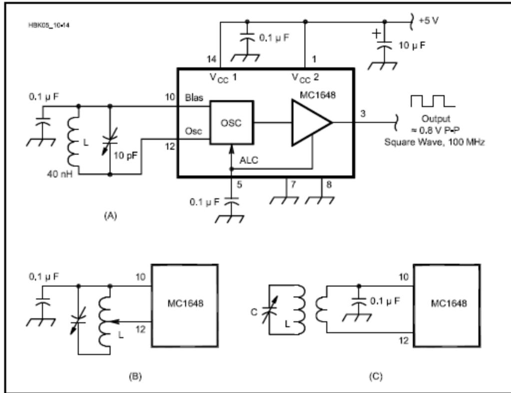
**Figure 1** — One of the few ICs ever designed solely for oscillator service, the ECL Motorola MC1648 (A) requires careful design to avoid VHF parasitics when operating at HF. Keeping its tank Q high is another challenge; B and C show means of coupling the IC's low-impedance oscillator terminals to the tank by tapping up on the tank coil (B) or with a link (C).
